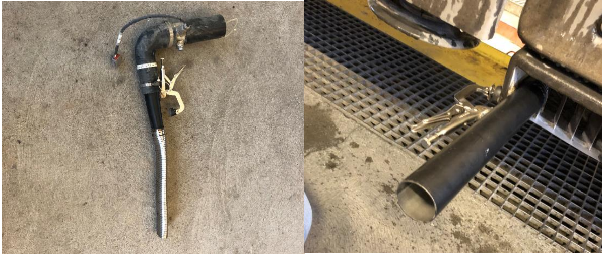
Figure 14. Special probe for exhaust outlets of the type as is shown to the right
