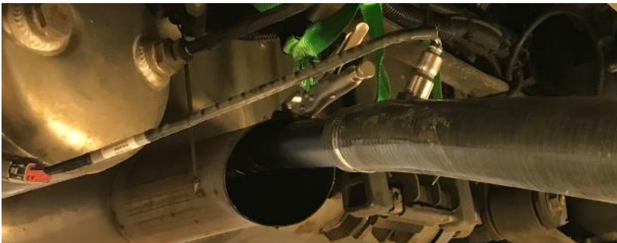
Figure 13. Test probe mounted in exhaust pipe
